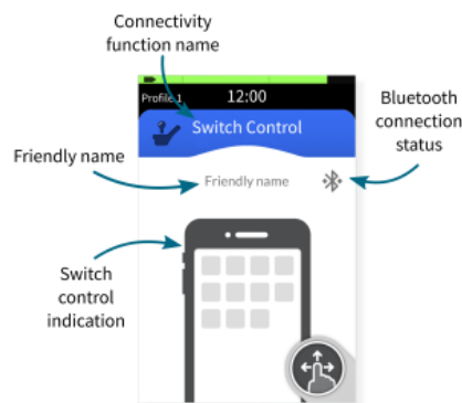
Figure 105 : Switch control components
