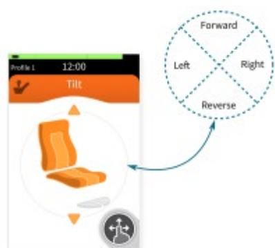
To show the user which movements are available and how to use them, the movements are displayed in one of the four dials (front, back, left and right) of the circular dial.
