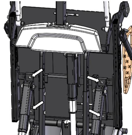
Figure 13 : Seat width adjustment
