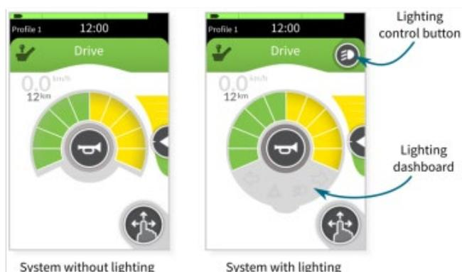
Figure 63 : Driving card with and without lighting
