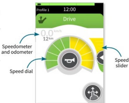
Figure 56 : Driving map showing speedometer/odometer, speed dial and speed slider
