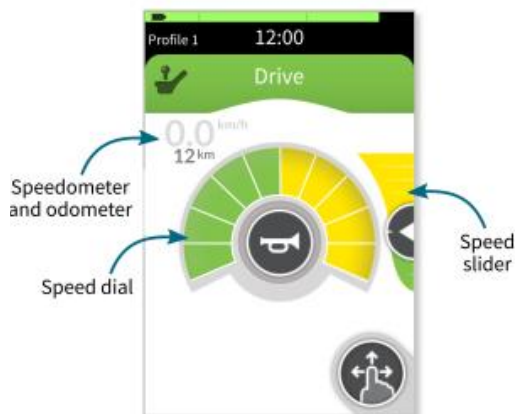
Picture56 : Drive card showing the speedometer/odometer, speed dial, and speed slider
