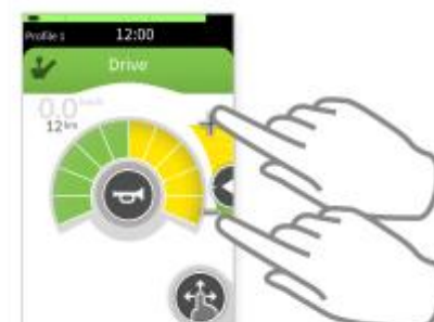
Picture61 : Adjusting the speed slider in tap-only mode
