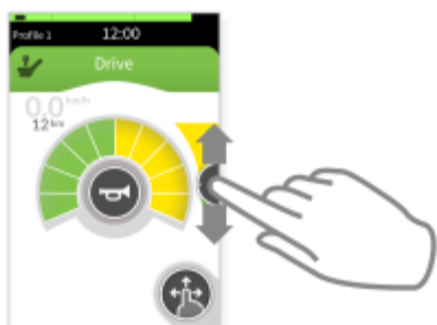
Picture60 : Adjusting the speed slider in touch-slide mode
